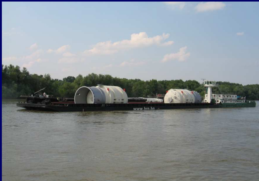
Transport of 2 x 550 mts Chemical Reactors from Degendorf to Transhipment at Port of Constanta to a heavy-lift vessel Constanta
