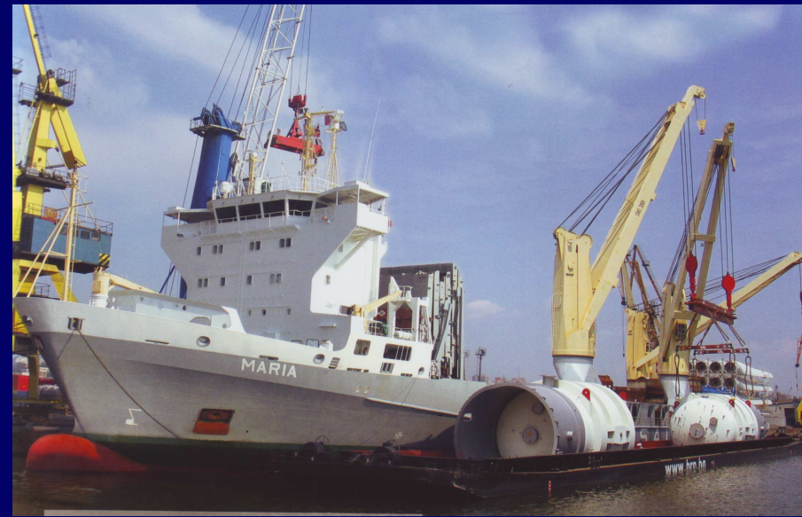
Transport of 2 x 550 mts Chemical Reactors from Degendorf to Transhipment at Port of Constanta to a heavy-lift vessel Constanta
