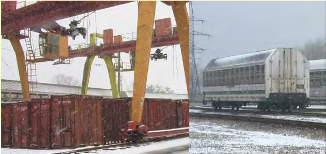
Figure 29: LISKI-Kiev – Gantry Crane and Specialised Wagon to Transport Cars
