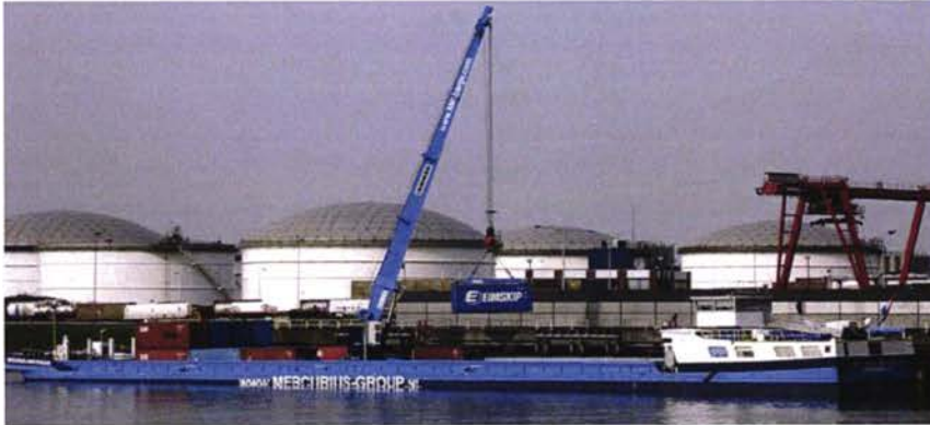
Figure 11.13 Container Barge with Crane
