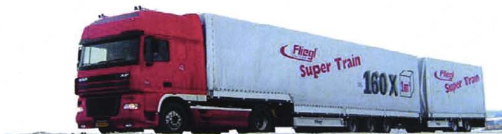
Figure 1. An articulated road-train of 25,25m long and body space of 160m 3 .
