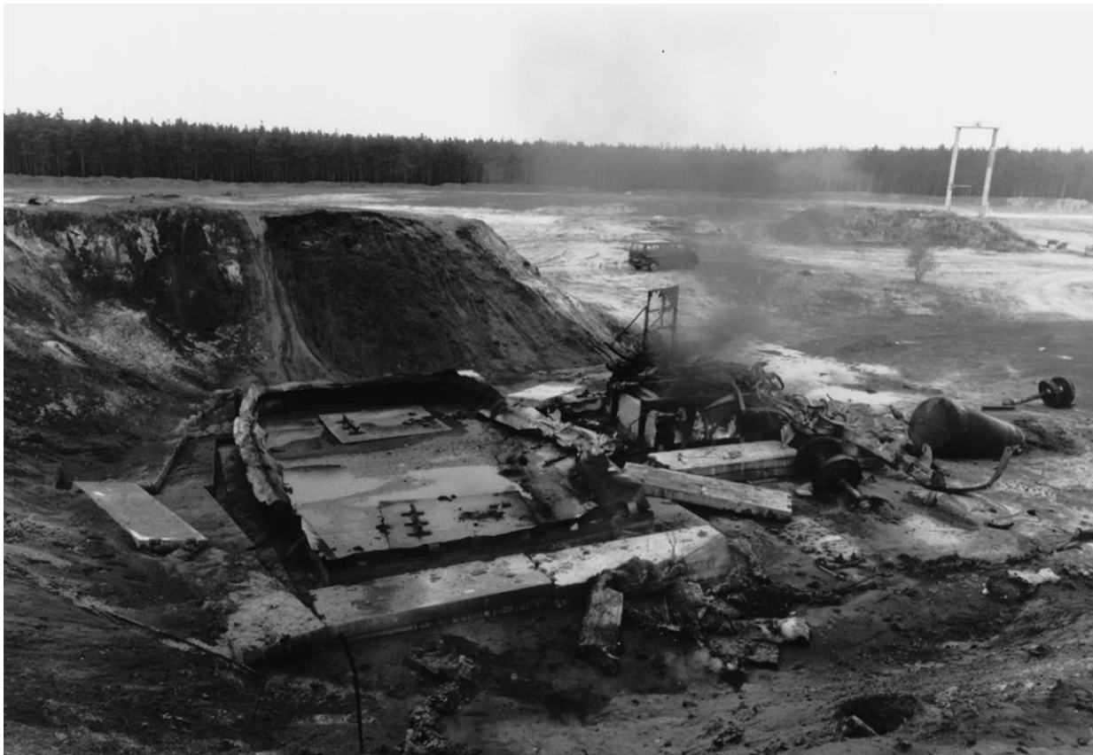
Picture 3.2 LPG rail tank car after the test.
