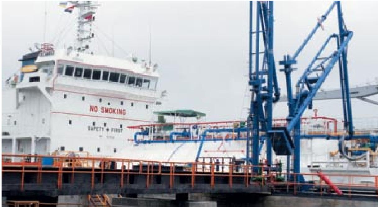
Figure 2.3 LPG vessel loading – special loading arm device
