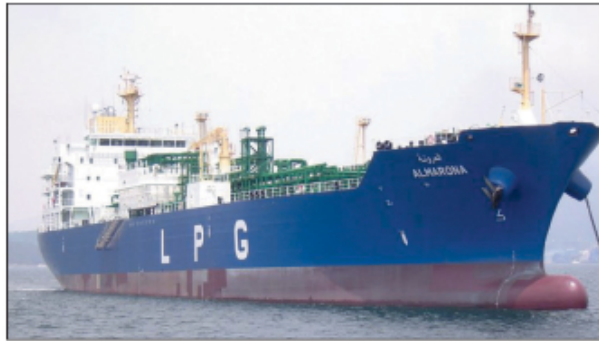
Almarona is the first of two new 23,000m 3 LPG tankers - the first of this type to be built by STX - for Qatar Shipping.
