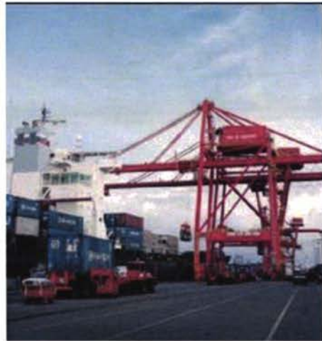
Ship-to-shore gantry cranes
