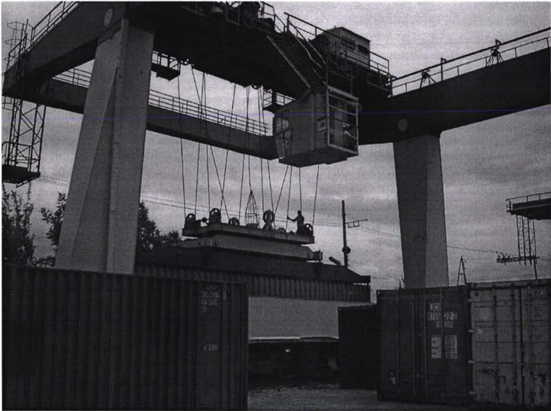
Figure 5 – Dushanbe terminal – Gantry crane lifting a 40’ container
