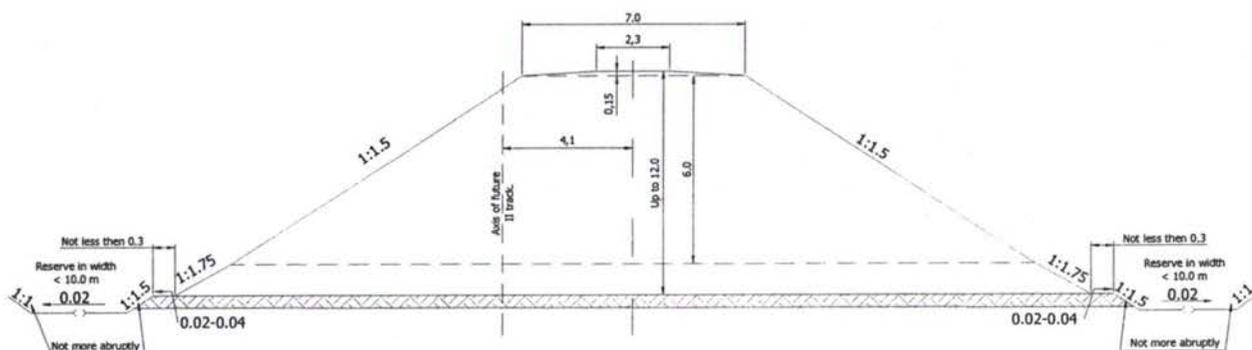
Typical cross structure of embankment in height up to 12 m from clay soils, fine and powdery sand and it is easy weathered rock.
