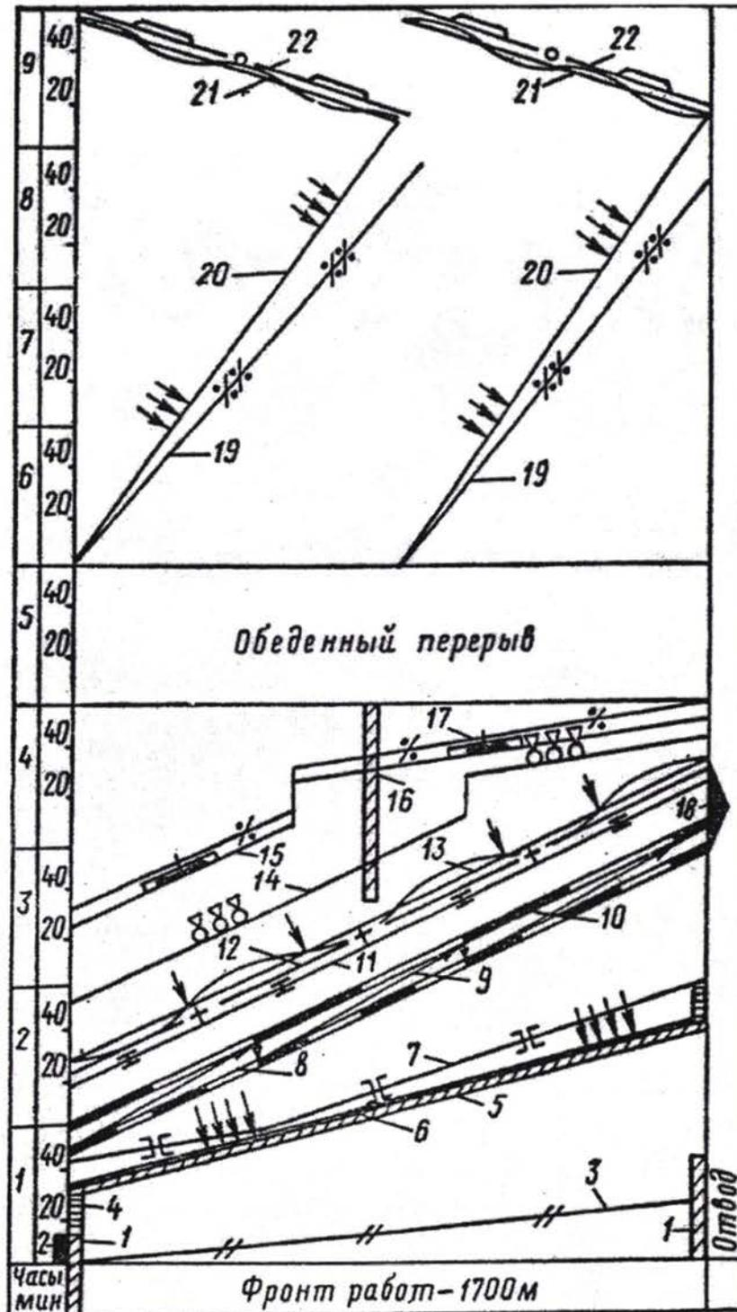
1 – preparing for charging and discharging of gravel-cleaning machine; 2 – securing the closure of the route section; 3 – preparing for dismantling; 4 - preparing for charging and discharging of gravel-cleaning machine; 5 – gravel cleaning; 6 – track rectification; 7 – unbolting the rail joints; 8 - dismantling of the track; 9 – gravel
