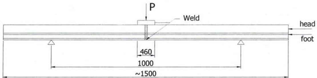
Load P shall be increased slowly from 0 to 40 tons, continuously recording the deflection of the mid portion. Under the maximum load neither cracks nor fractures shall appear. After removing the load, the residual permanent deformation shall be measured one hour after the test.
