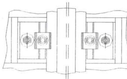
Normally rails are provided in 25 m bars; so, when they are laid down, a joint has to be done every 25 m. To reduce the hammering at the passage of trains, the joints on one rail are displaced 3 cm from the relevant ones on the other rail along the track
