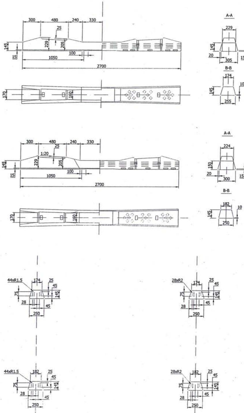
Design of ferroconcrete sleepers
