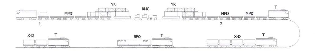
1 - dismantling (distributor) train; 2 - packing (laying) train; T - disel locomotive; MPD - motor platform; YK - laying crane; BMC - balast dearer; XD - hopper-batcher; BPO - liner-tamper supfaser. TITALFERR
