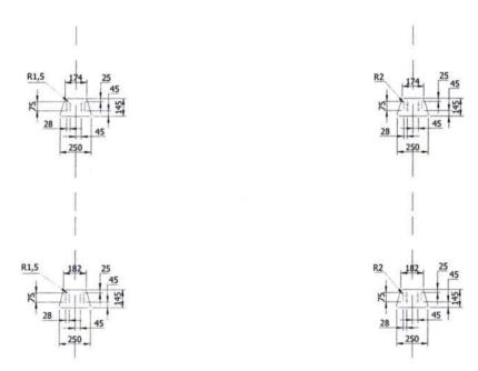
Design of ferroconcrete sleepers a - such as C-73-1; b - such as C-73-2; c - cross sections and reinforcing of sleepers C-73-1; d - cross sections and reinforcing of sleepers such as C-73-2.
