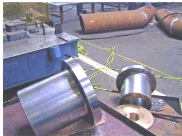
Propulsion shaft couplings
