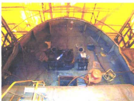
View from wheelhouse to forecastle with anchor windlass
