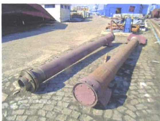
Sterntubes ready for installation
