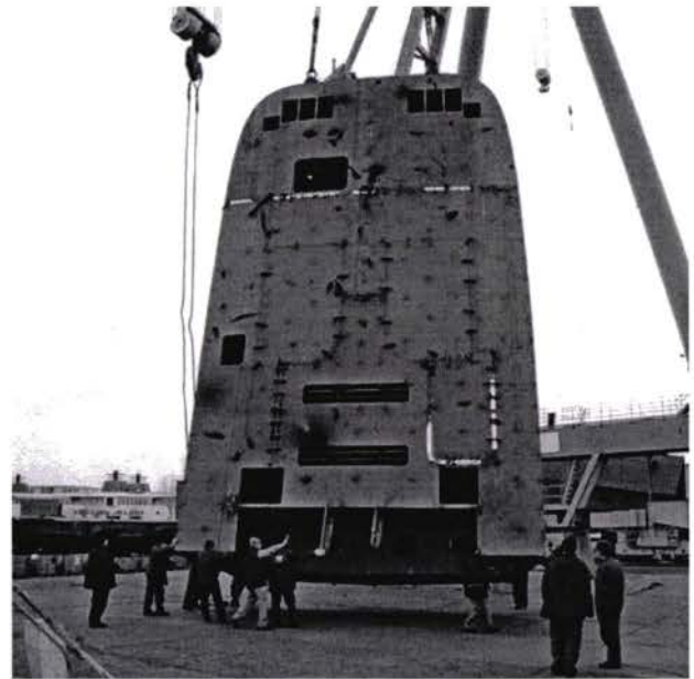
Main deck of aft section during turning
