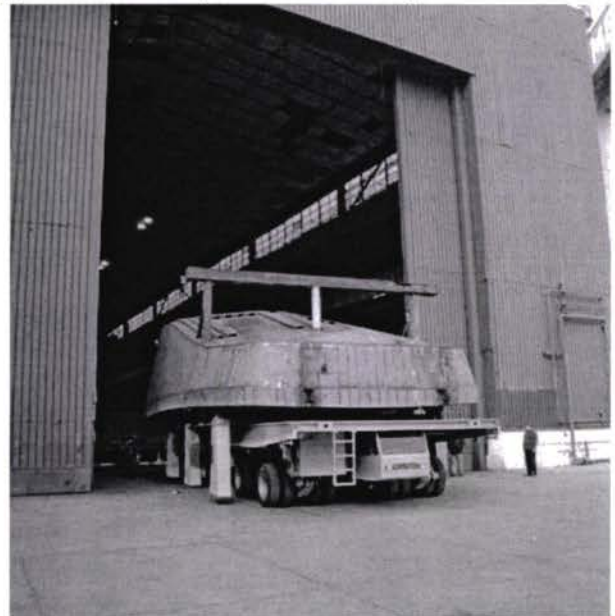
Aft Section on the way to slipway for turning
