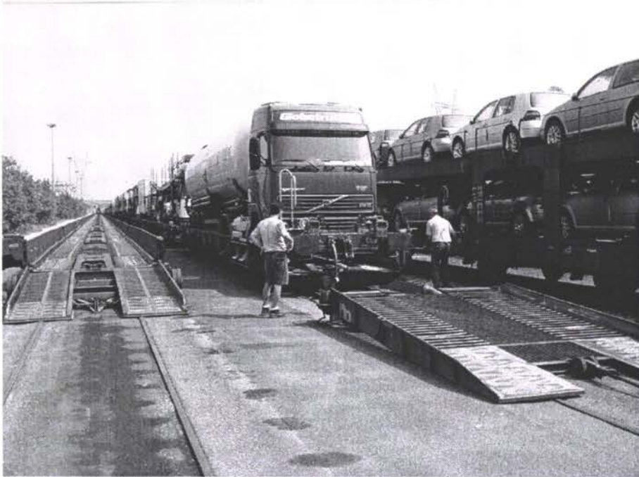
ROLA Train at Verona showing ramp about to be positioned
