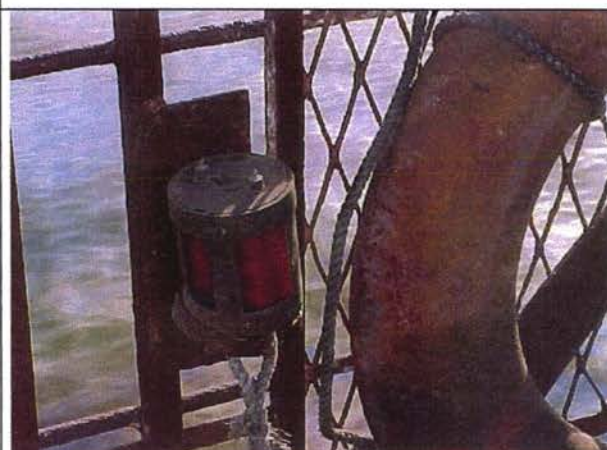
Life-belt, without name and homeport, cover broken and not watertight, light without battery, socket and bulb
