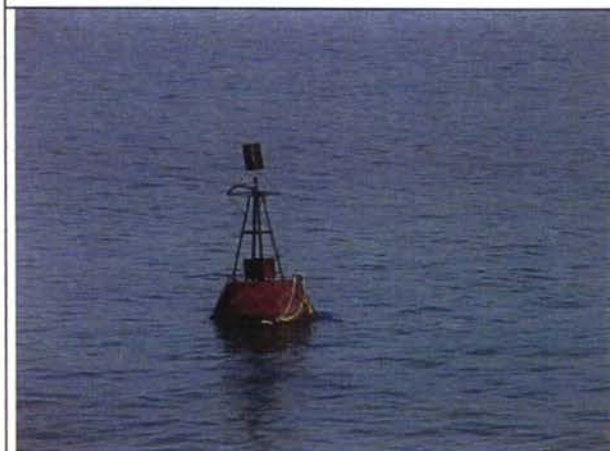
Buoy without radar reflector, colour must be red -not recognizable
