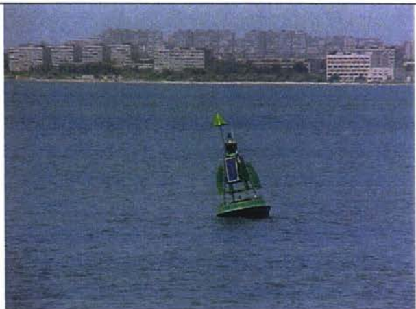
Starboard buoy with radar reflector, sun collector and light
