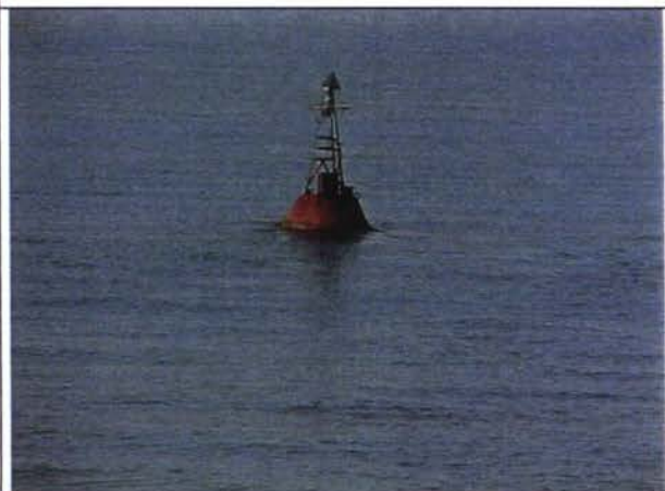
Buoy without radar reflector, colour must be green or black - not recognizable
