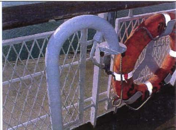
Life-belt and emergency lamp construction without socket and bulb
