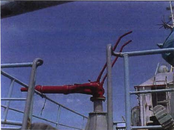
Monitor for water and foam on the garbage, sewage and oily water boat "Raduga"
