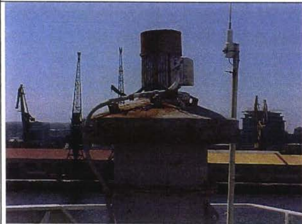
Ventilator for passenger cabins, cable broken
