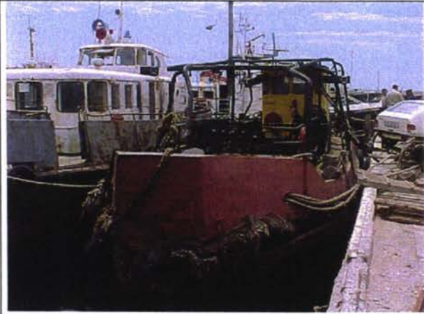
Vessel for collecting oily water and garbage
