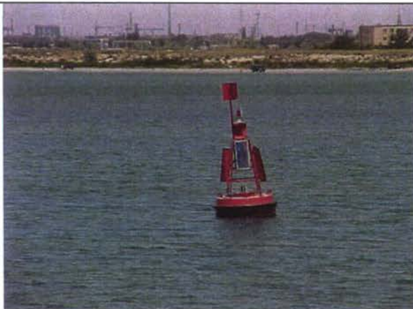
Fair way buoy with radar reflector, sun collector and light
