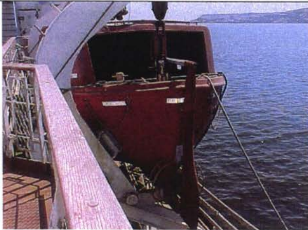
Life boat starboard side, 52 persons, bad condition, but useable
