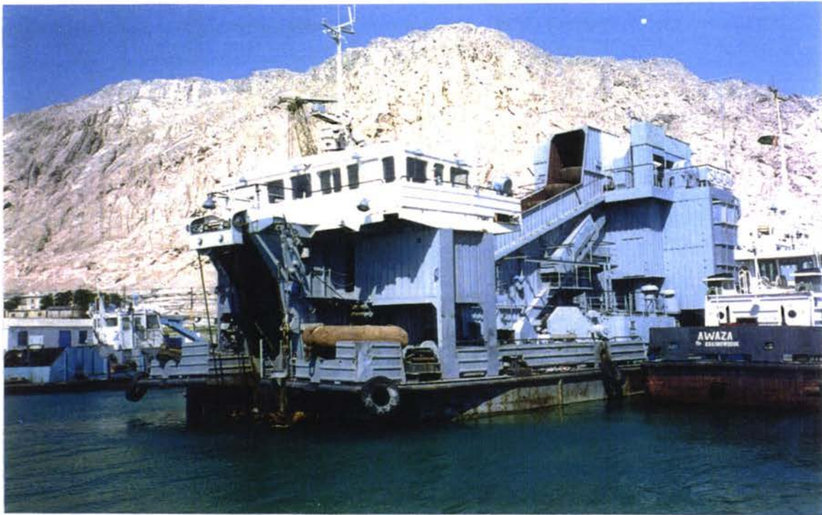
1. Bucket dredger in Turkmenbashi harbour
