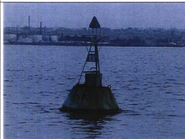
Buoy 13 is green painted, since it is dividing the channel it must be green-red-green coloured
