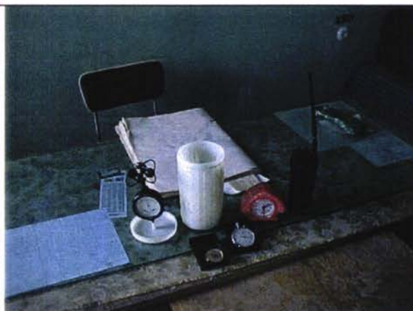
Equipment of the Port Control Centre Dubendi, wind speedometer with container, alarm clock, wristwatch without bracelet, stopwatch log book and hand held radio with only VHF and limited channels
