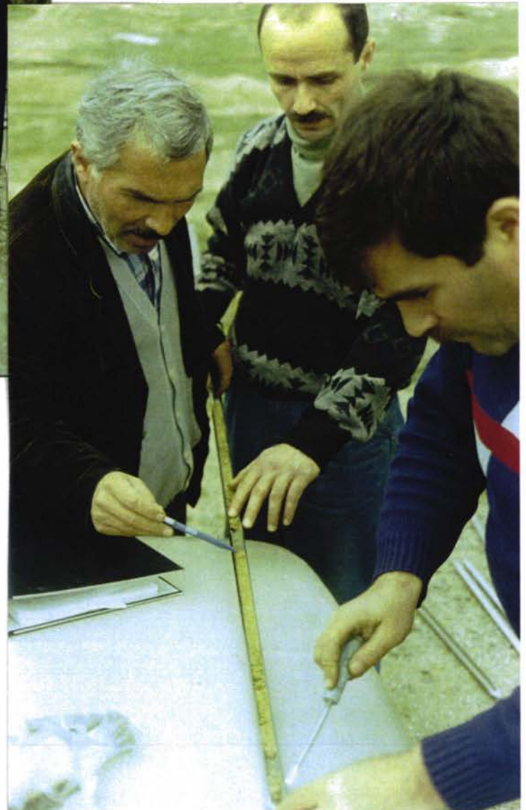
Drill sounding, analyse of extracted soil sample
