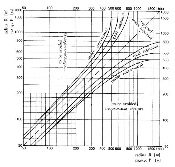
Length of straight Road Section and minimum Radius of Curve after straight Road Section
