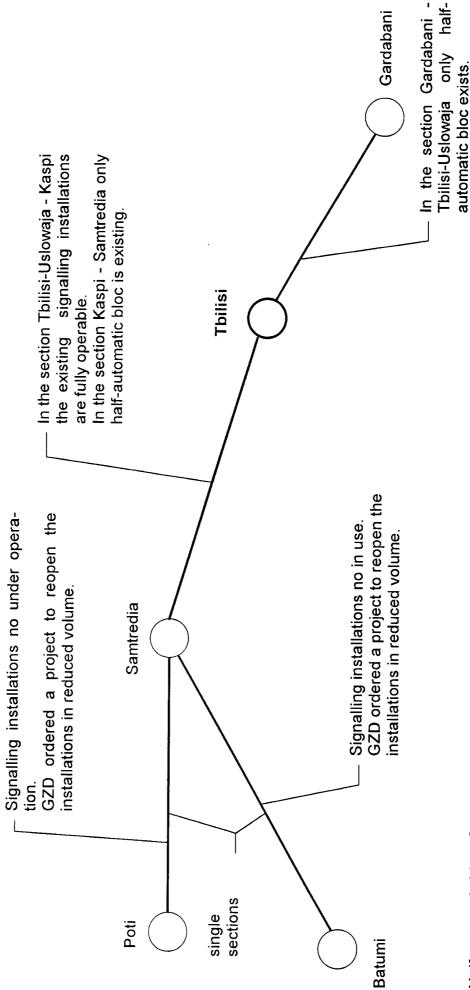
Half-automatic bloc: Operation only in bloc distance from station to station.
