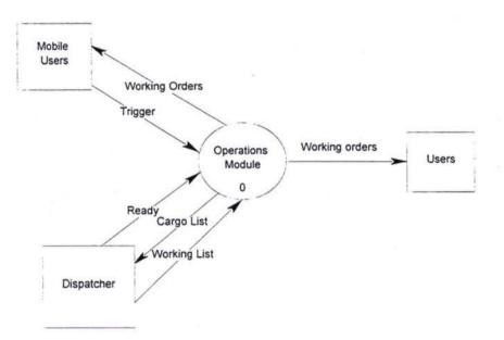
The above context diagram shows merely that the dispatcher makes the working list and the user of the mobile terminals or other users can work with this list.
